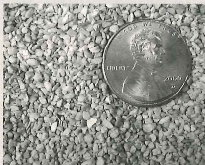
Figure 1 - Corn cob media used in lautertun
